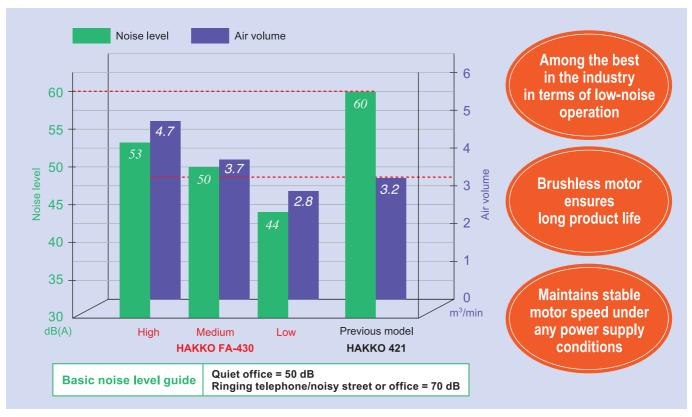
Notes regarding graph: The HAKKO FA-430 features significantly reduced noise level in medium airflow mode despite the fact that suction performance remains almost unchanged compared to the previous model. High airflow mode also provides quieter operation than the previous model.
